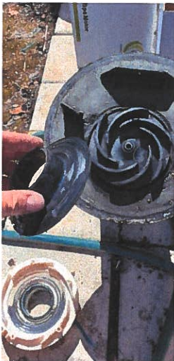
Separated impeller and damaged diffuser, main seal plate in background also damaged.
